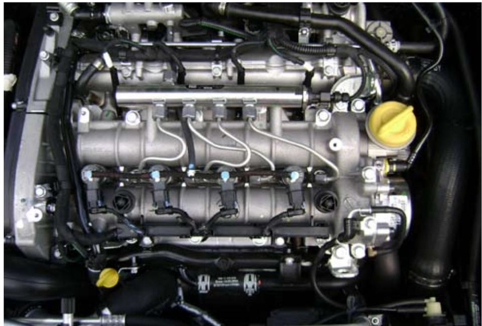
*Vauxhall Vectra 1900cc Common Rail Diesel – under the bonnet (cover removed)*
