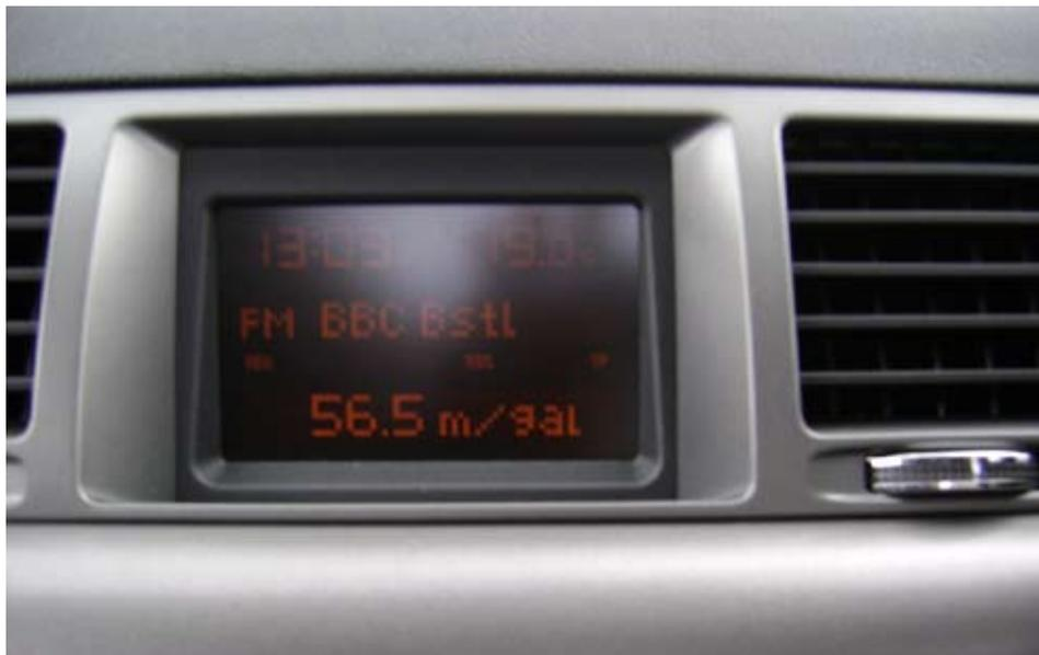
*Instant fuel consumption figure which is equal to 5 litres per 100kms at 110km/h Vauxhall Vectra 1900cc Common Rail Diesel*
